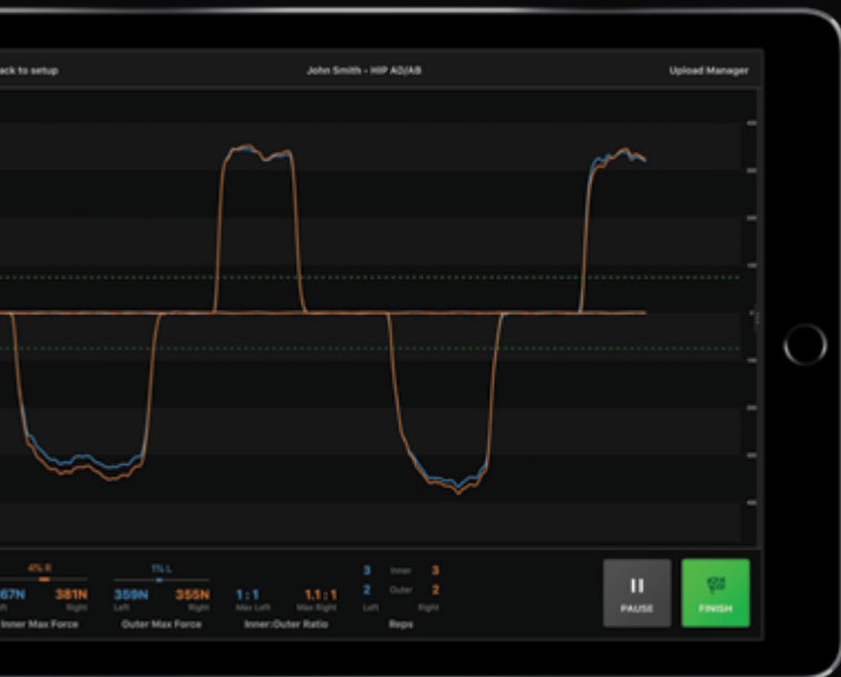
Live graphing of the force trace shows strength in newtons
